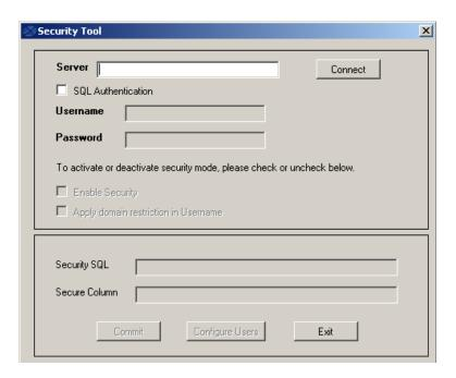
4. In the Server field, type in the Server name and, if applicable, the instance name for the SQL Server that hosts the SQL metadata databases (BizInsight and BizInsightDB). The connection will be made using Windows Authentication by default. Check the SQL Authentication checkbox to switch to SQL credentials and supply those credentials in the Username and Password fields. Click Connect.
